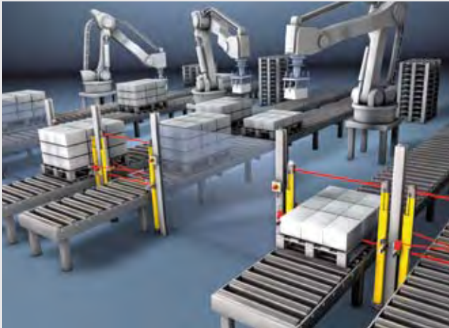
MLD 500 Multiple Light Beam Safety Device with integrated Muting indicator in an application with parallel Muting.
