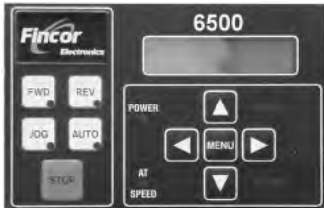
FIGURE 3. OPERATOR PANEL FOR SERIES 6500 CONTROLLERS
