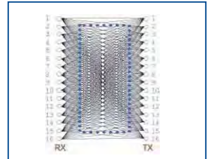
SCAN MODE 3-4: low speed / high resolution Minimum object detection Flat = 0.2 (thickness) x 75 (width) mm Cylindrical objects = Ø 6 mm
