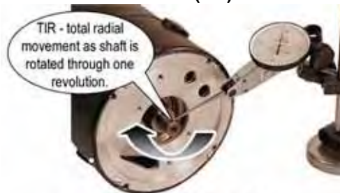
Figure 3 - Total Indicated Runout
